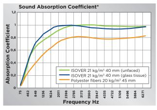
\*Sound Absorption Coefficient according to ISO 10534-2
