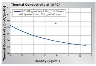
\* Thermal Conductivity at 10°C according to EN 12667
