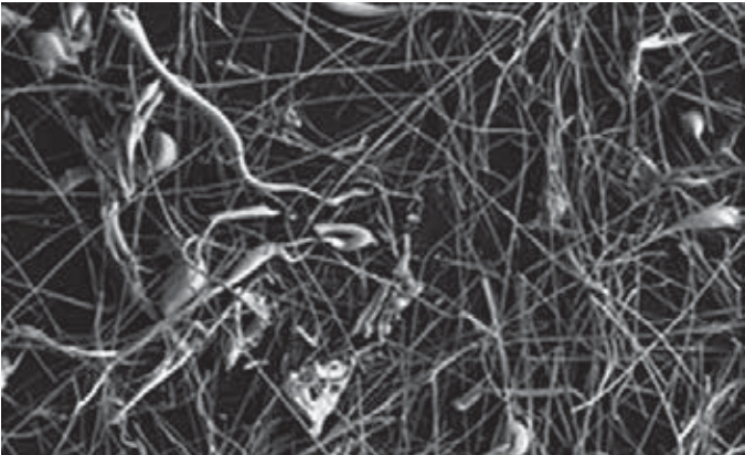
Traditional stone wool microstructure (25 % - 40 % of slugs/ unfiberized particles)
